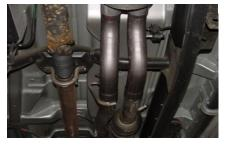
SLIDE PASSENGER SIDE HEADPIPE #A ONTO STOCK HEADPIPE. INSERT WELDED HANGER INTO RUBBER GROMMET. NEXT INSTALL DRIVERS SIDE HEADPIPE #B ONTO STOCK HEADPIPE, USE CLAMP #G TO SECURE BOTH HEADPIPES, DO NOT TIGHTEN.
