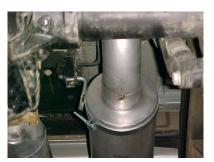
NEXT, INSTALL BAND CLAMP # H ONTO MUFFLER INSERT HANGER INTO RUBBER GROMMET. USE BOLT KIT PROVIDED FOR BAND CLAMP, DO NOT TIGHTEN.
